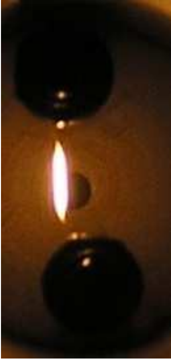
Figure 3. A photograph of the 5 \mu\text{m} diameter wire with 10 mA current flowing through it. The two black circles on the upper and lower ends are the feedthroughs.
