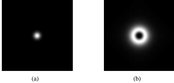
FIG. 2: Intensity profile at the exit face of the 1-plate. (a) Full SAM-to-OAM conversion; (b) No SAM-to-OAM conversion.
