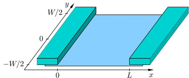
FIG. 1: (Color online) Schematic setup for two-terminal transport measurements. Graphene sample of dimensions  $L \times W$  is placed between two parallel contacts. We assume  $W \gg L$  throughout the paper.
