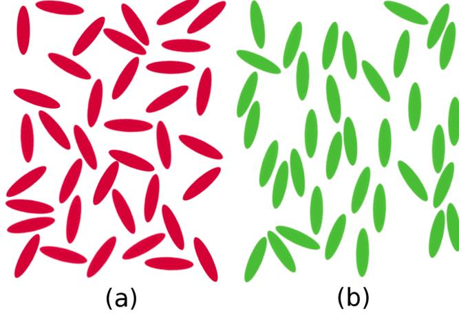
Figure 4: (Color online) schematics of the a) isotropic and b) uniaxial nematic phases with rod-like mesogens.
