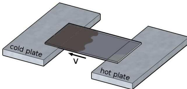
Figure 1: Schematic of a directional growth experimental system where a slide/thin film enclosing a material is pulled at a constant velocity  $v$  from a plate or oven at a temperature above the phase transition temperature to one that is below the phase transition temperature; the opaque portion of the slide represents the ordered/solid phase and the translucent portion represents the disordered/liquid.
