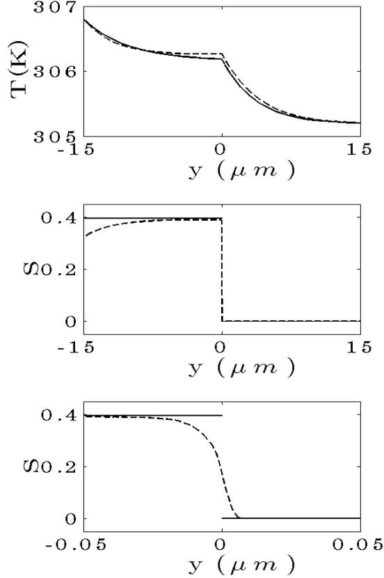
Figure 6: Sample order parameter and temperature profiles for initial flat interfaces from the sharp-interface model (solid lines) and stationary simulation results (dotted lines) a) (top) temperature versus y-coordinate over full domain b) (middle) uniaxial nematic scalar order parameter versus y-coordinate over full domain c) uniaxial nematic scalar order parameter versus y-coordinate magnified in the interface region.
