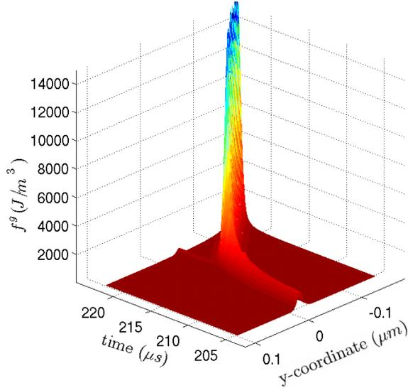
Figure 11: (Color online) Surface plot of the gradient free energy density (refer to Eq. (3)) as a function of time and y-coordinate ( $\mu m$ ); features of the energy surface include the initial homeotropically oriented interface, defect shedding (the high energy peak), and the relatively lower energy planar oriented interface.
