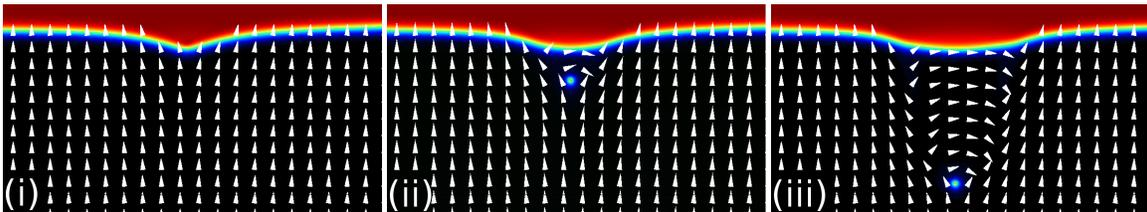
Figure 9: (Color online) initially homeotropic defect formation i)  $t = 214.5\mu s$  ii)  $t = 219.4\mu s$  iii)  $t = 229.1\mu s$ ; the surface corresponds to the scalar uniaxial nematic order parameter (red/black corresponds to isotropic/nematic), arrows correspond to the uniaxial nematic director (should be considered headless), and horizontal length scale is  $0.65\mu m$
