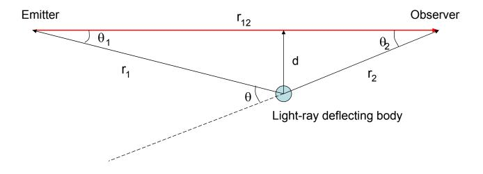
**Figure 1.** Ranging time delay experiment. Electromagnetic signal is emitted at distance  $r_1$  from the massive body, passes by it at the minimal distance d, and is received by observer at distance  $r_2$ . The emitter, observer, and the massive body move with respect to each other as the electromagnetic signal propagates. This makes the ranging delay experiment sensitive to the null cone structure of space-time in general relativity and modifies the Shapiro time delay.
