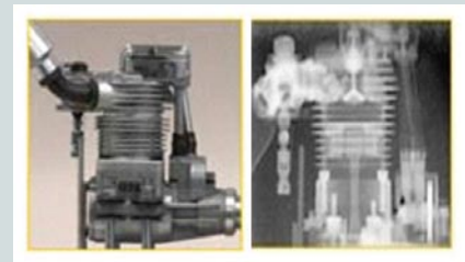
A 150-cc model airplane engine (left), and a proton radiograph of it produced using 800 MeV protons (right). The details of the thicker parts of the engine are clear in the proton radiograph.
