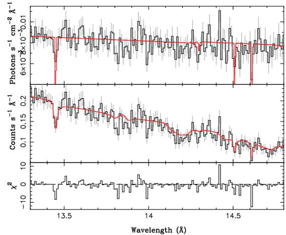
FIG. 5.— Flux corrected spectra (top panel) and count rate per angstrom (middle panel) for the combined MEG  $\pm 1^{\text{st}}$  order spectra, with an absorbed `diskbb` model fit in the 13–15 Å region (see text). The top and middle panels show the data fit with the Ne II, Ne III, and Ne IX lines, while the residuals show a fit without the lines.
