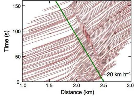
Figure 4: Measured vehicle trajectories due to J. Treiterer. The green line shows the experimental measurement of [2] (Figure reproduced from [2] with permission).
