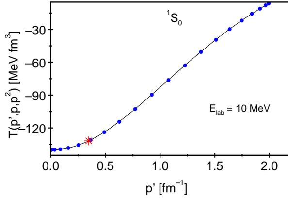
Fig. 20: (Color online) Comparison of the half-on-shell  $T(p', p, p^2)$  matrix elements (continuous line) with those of  $T_{\text{low-k}}(p', p, p^2)$  for  $p = 0.35$  fm $^{-1}$  ( $E_{\text{lab}} = 10$  MeV). The asterisk indicates the on-shell matrix element. The cutoff momentum is  $\Lambda = 2$  fm $^{-1}$ .
