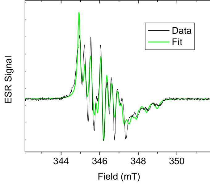
**FIG. 4 (color online).** ESR spectrum of Sc@C<sub>82</sub> at 80 K in frozen solution. The data were fitted using the  $g$ -tensor and hfs-tensor given in Equations (2) and (3). The slight change in resonant field compared with Fig. 3(a) arises from retuning the microwave frequency following the change in the cavity temperature.
