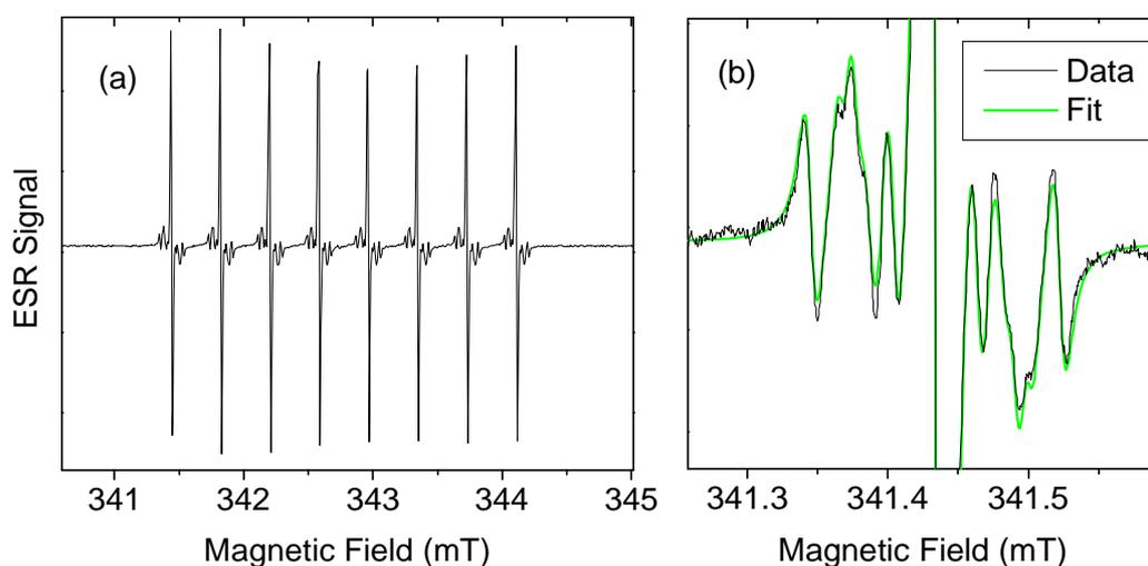
**FIG. 3 (color online). Room temperature CW-ESR spectra of  $\text{Sc@C}_{82}$ : (a) full spectrum; (b) enlargement of lowest-field line, with the best fit using five Lorentzian curves in grey (green online), using the hfs constants in Table II.**
