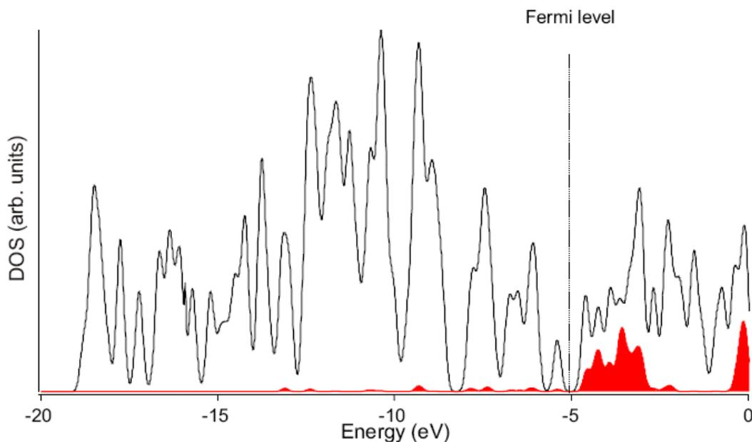
**FIG. 5 (color online).** The calculated total DOS (curve) and Sc PDOS (solid area, red online) of Sc@C<sub>82</sub> by ADF code [15]. Gaussian bands of 0.25 eV half-width were used. The solid area at energies lower than the Fermi level corresponds to the 2.09 electrons in the 3d, 4s, and 4p orbitals of the Sc atom.
