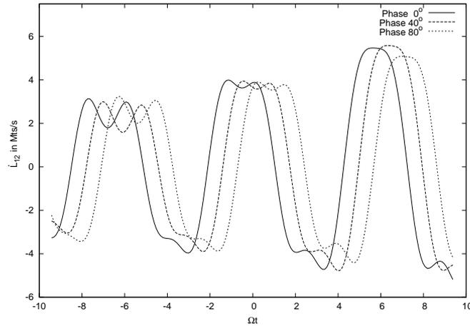
**Figure 3.** The figure shows the flexing of the arm  $l_{12}$  for the different phases  $t_0 = 0, 40^\circ, 80^\circ$  and  $-3\pi \leq \Omega t \leq 3\pi$ . The maximum flexing is seen to be insensitive to the phase.
