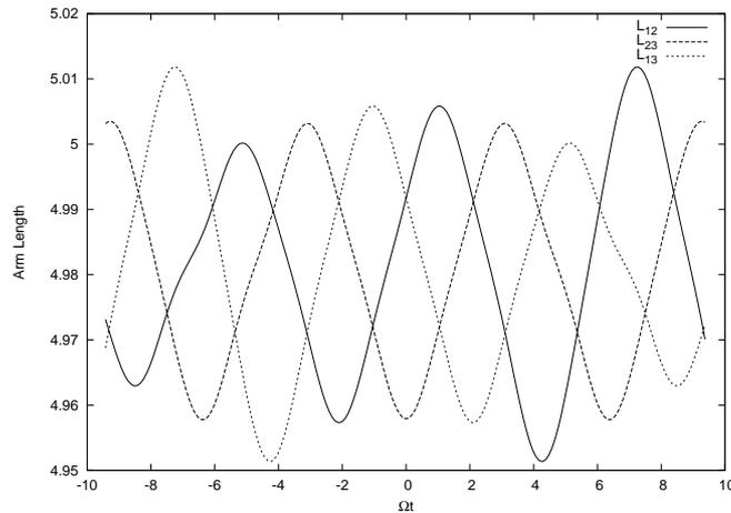
**Figure 1.** The figure shows the variation in the three armlengths of LISA for a mission period of three years ( $-3\pi \leq \Omega t \leq 3\pi$ ) for the phase  $t_0 = 0$  in millions of km. The maximum variation in armlengths is about 60,000 km.
