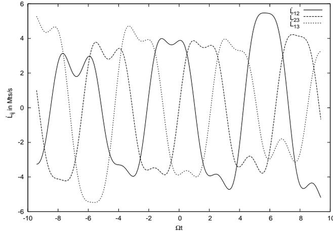
**Figure 2.** The figure shows the time derivative of the armlengths for a mission period of three years ( $-3\pi \leq \Omega t \leq 3\pi$ ) for the phase  $t_0 = 0$ . The flexing of the arms is less than 5.5 metres/sec.
