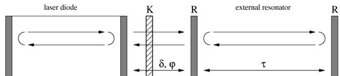
FIG. 1: Schematic diagram of a semiconductor laser with resonant feedback from a Fabry-Perot resonator.  $K$  denotes an attenuator,  $R$  is related to the mirror reflectivity of the external resonator,  $\tau$  is the round trip time of the resonator,  $\varphi$  and  $\delta$  are phase shift and latency time due to the distance between laser and resonator.
