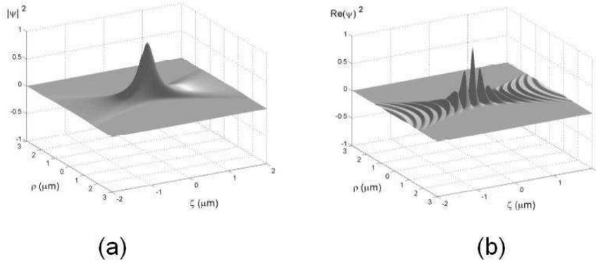
Figure 3: **(a)** and **(b)** show, respectively, the intensity of the complex and real part of an ultrashort, totally “forward”, superluminal FWM optical pulse, with  $V = 1.5 c$ ,  $\alpha_0 = 1.256 \times 10^7 \text{ m}^{-1}$  and  $s = 2.3873 \times 10^{-7} \text{ m}$ , which correspond to  $\omega_{\min} = 3.77 \times 10^{15} \text{ Hz}$ , and  $\Delta\omega = 1.88 \times 10^{15} \text{ Hz}$ , i.e., to a femtosecond optical pulse.
