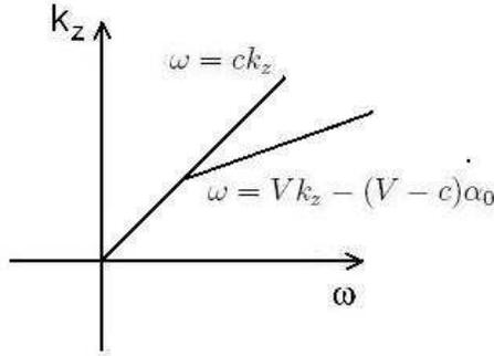
Figure 1: The Dirac delta function in (13) confines the spectral parameters  $\omega, k_z$  of the Bessel beams to the straight line  $\omega = V k_z - (V - c)\alpha_0$ , with  $\alpha_0 > 0$ .
