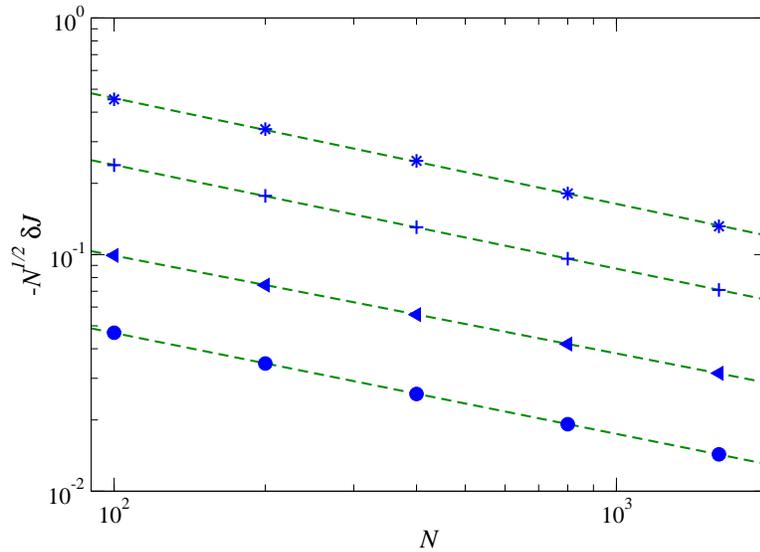
**Figure 3.** Finite size deviation of the heat flux  $\delta J \equiv J - J_{num}$ , rescaled by  $N^{1/2}$ , as a function of the size of the chain  $N$ , for  $\gamma = 1$  (circles), 2 (triangles), 5 (pluses) and 10 (stars), other parameters as in the previous figure. The lines correspond to power-law fits, from which we extract that the corrective terms scale as  $-\delta J \sim N^{-\alpha}$  with  $\alpha = 0.927, 0.914, 0.939$  and  $0.947$ , respectively.
