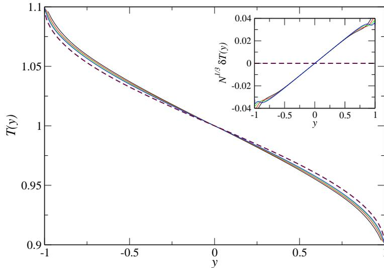
**Figure 2.** Temperature profile  $T(y)$  as given by the analytical expression (18), for  $T_+ = 1.1$ ,  $T_- = 0.9$ ,  $\omega = \lambda = \gamma = 1$  (dashed curve). The solid curves correspond to the profile  $T_{num}$ , obtained from the numerical solution of equations (16a-16c) for  $N = 100, 200, 400, 800$ . The finite-size deviations from (18),  $\delta T \equiv T - T_{num}$ , rescaled by  $N^{1/3}$ , are shown in the inset.
