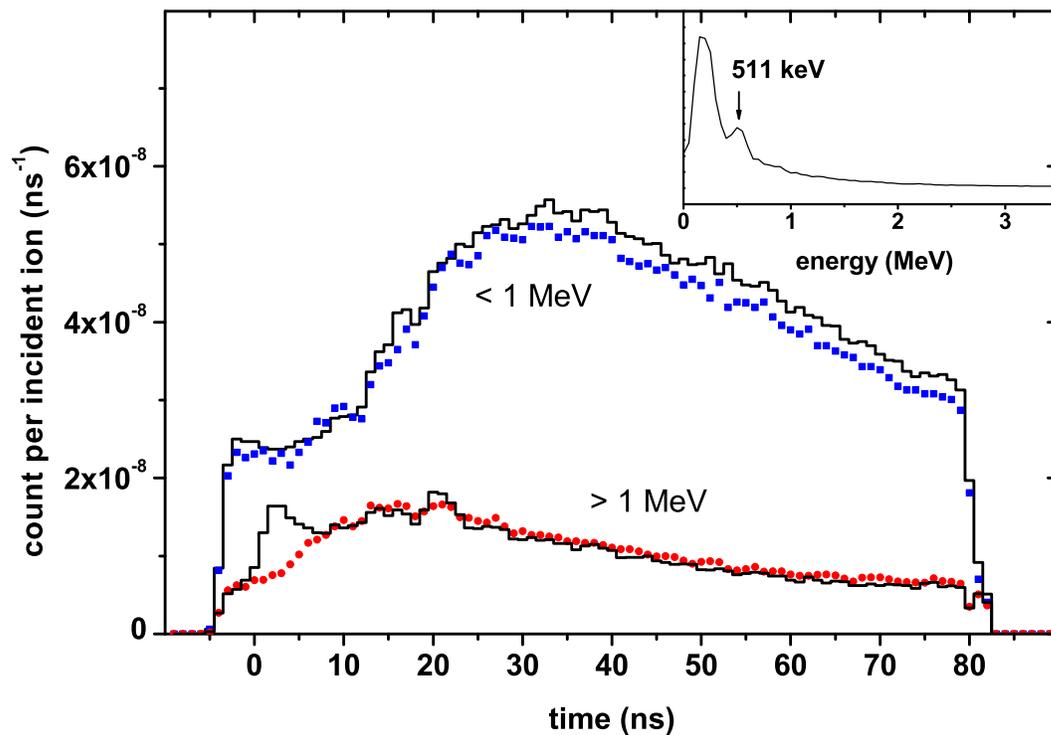
FIG. 2: Time-of-flight spectra measured for two target locations  $Z$  and for two selections on energy  $E$  deposited in scintillator :  $Z = 8$  mm (lines),  $Z = 26$  mm (dots),  $E < 1$  MeV and  $E > 1$  MeV. Origin of time scale: ion impact on target. Inset: measured energy spectrum.
