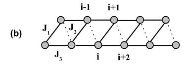
FIG. 1: Diagram of the  $J_1 - J_2 - J_3$  model which can be considered either as a linear chain(a) or a zigzag chain(b). The alternating nearest-neighbouring interaction is  $J_1$  and  $J_2$  respectively, while the next-nearest-neighbouring interaction is parameterized by  $J_3$
