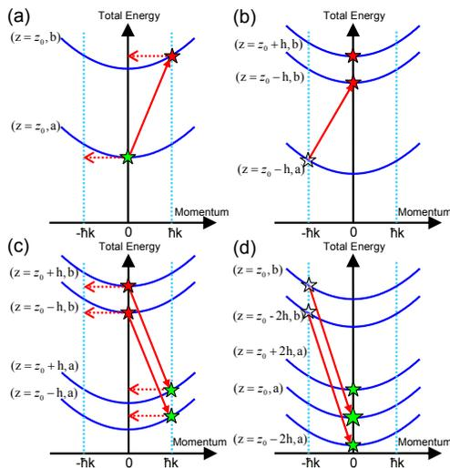
FIG. 4: Motion of the atomic wave-packets in the energy-momentum picture for the interferometer duration  $2T^0$ . Figs. (a,b,c,d), associated with the 1st,2nd,3rd and 4th light pulses respectively, show the packets present in coherent superposition (full stars) immediately after - or transferred (transparent stars) during - the considered pulse, whose effect is represented by a full red arrow.
