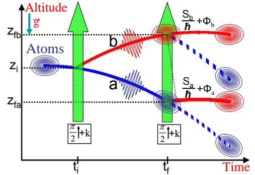
FIG. 1: Action of two distinct  $\pi/2$  pulses on a free-falling atomic wave-packet. The phase difference between the two outgoing wave-packets comes from the classical action and laser phase acquired on each path, and from the distance of their centers.
