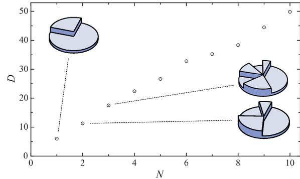
FIG. 3: (color online). Maximum dimensionality that can be accessed with sector phase plates having  $2N$  angular sectors alternatingly phase shifted by  $\pi$ . The insets show the optimized plates for  $N = 1$ ,  $N = 2$  and  $N = 3$ .
