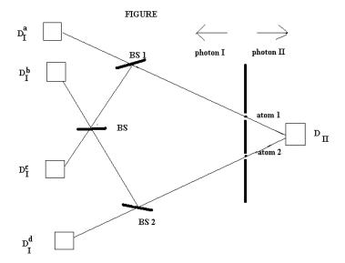
Figure 1: The two-photon 'two-slit' random-choice and delayed-choice erasure experiment outlined in section 2.
