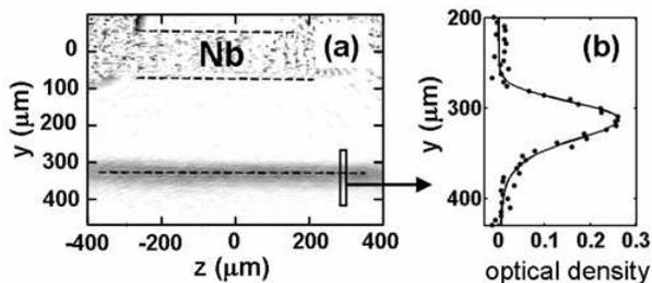
FIG. 3: (a) Absorption image of the atomic cloud at the central region of the magnetic trap. The dashed lines represent the longitudinal axis of the trap, and the Nb wire surface. (b) Optical density of one of the transverse sections of the atomic cloud. The best-fit curve  $\rho(y)$  is also plotted.
