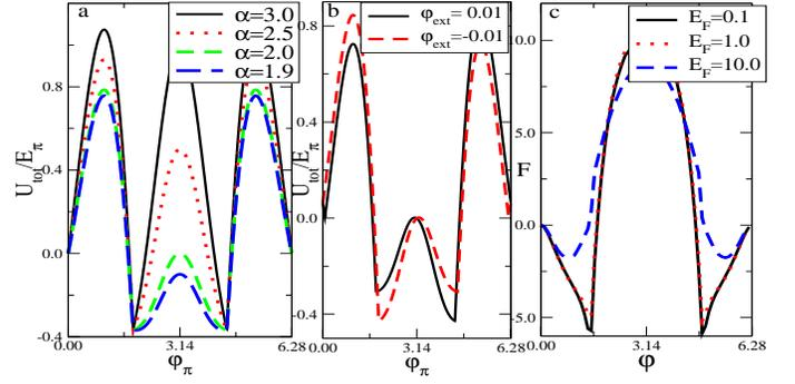
FIG. 4: (Color online) (a) Normalized energy,  $U_{tot}/E_\pi$ , as function of  $\phi_\pi$  for no external magnetic flux. (b) In presence of an external magnetic field with  $\alpha = 2.5$ . (c) The degenerate ground states of a d-wave Josephson junction.
