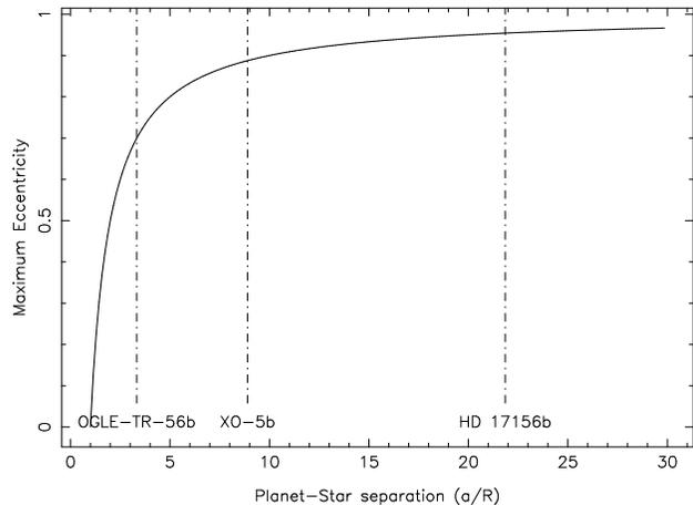
FIG. 5.— The maximum orbital eccentricity,  $e_{\max}$ , plotted as a function of the planet-star separation in units of  $a/R$  (see Equation 7) in order for a planet to remain outside the surface of its parent star. This requirement is purely based on system geometry and does not take into account tidal effects or planet-planet interactions, but requires that  $a > R$  when  $f = 0$ . Dot-dashed lines indicate values for  $a/R$  for various transiting planets.
