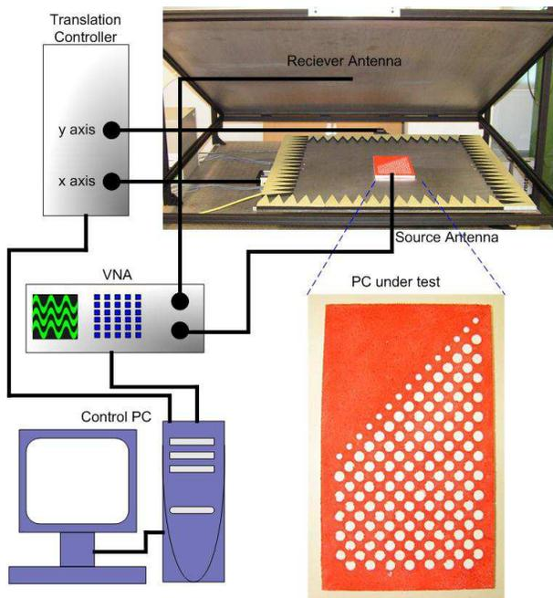
FIG. 2: (Color online) Experimental setup. Included are photographs of the parallel-plate waveguide mounted on a two-axis translation stage and the fabricated photonic crystal.
