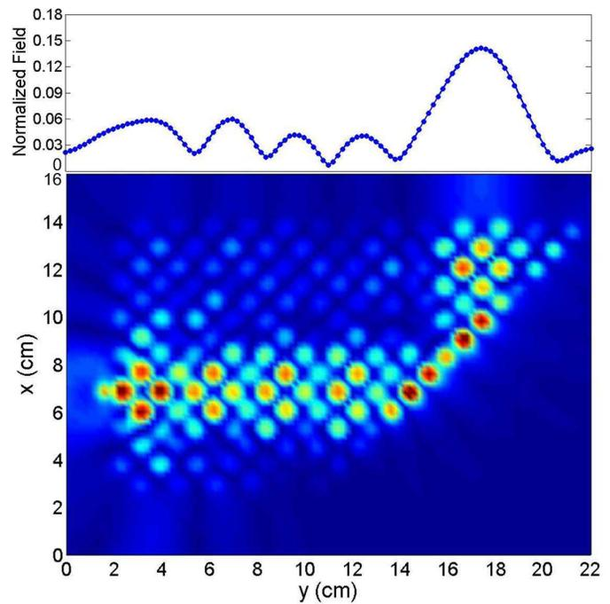
FIG. 3: (Color online) Experimental beam propagation in the photonic crystal of  $7.99\text{mm}\pm 0.02\text{mm}$  rods at the self-collimation frequency ( $7.64\text{GHz}$ ) reflected from the surface of  $5.92\text{mm}\pm 0.01\text{mm}$  rods. The measured GH is approximately 4 lattice spacings. Upper plot shows the output field taken one lattice period beyond the surface.
