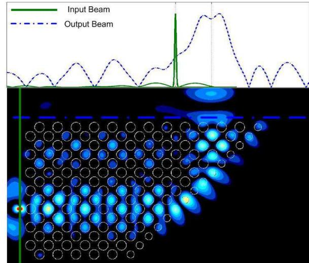
FIG. 1: (Color online) Numerical FDTD simulations of a reflected self-collimated beam experienced a GH shift for the modified surface of 5.92mm rods. Top: input (green) and output (blue) normalized field profiles. Bottom: Electric field generated by a point source and reflected by the surface.
