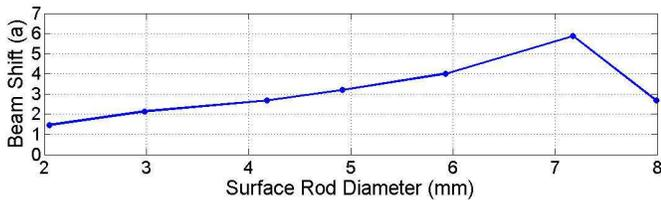
FIG. 4: (Color online) The experimental GH shift (measured in lattice periods) for a set of different surface rods. The maximal shift occurs for a small reduction in the diameter of the surface rod ( $7.175\text{mm} \pm 0.015\text{mm}$ ) and the smallest shift occurs for a large reduction in the surface rod diameter ( $2.005\text{mm} \pm 0.015\text{mm}$ ).
