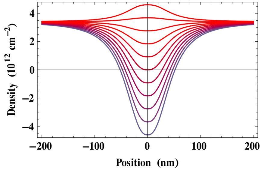
FIG. 4: Density profiles for  $V_{BG} = 50$  V over a range of top gate voltages (from eq. 8). Top gate voltage in 1 V increments. The width of the central region ( $L$ ) depends strongly on applied voltage.
