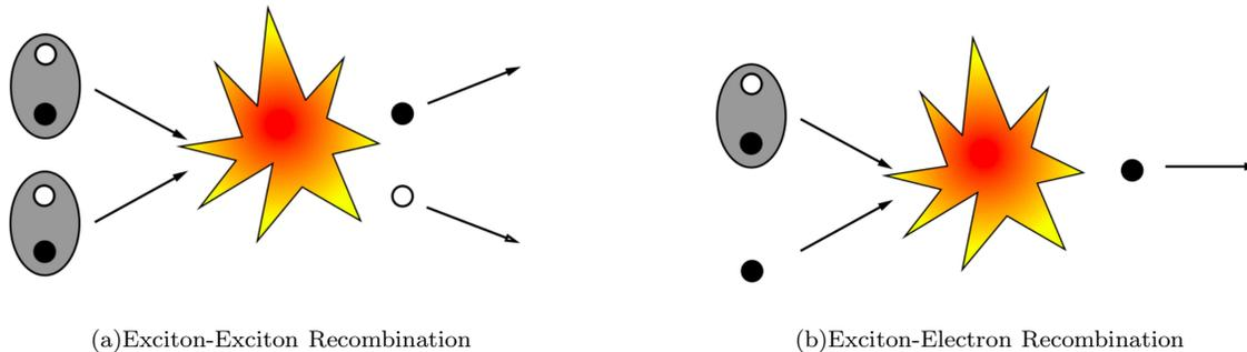
FIG. 1: (Color online) Schematic of two types of nonradiative Auger processes. In exciton-exciton recombination, a particle and a hole recombine and transfer their energy and momentum to the outgoing particle-hole pair. In exciton-electron recombination, all of the energy and momentum are transferred to a single outgoing particle.
