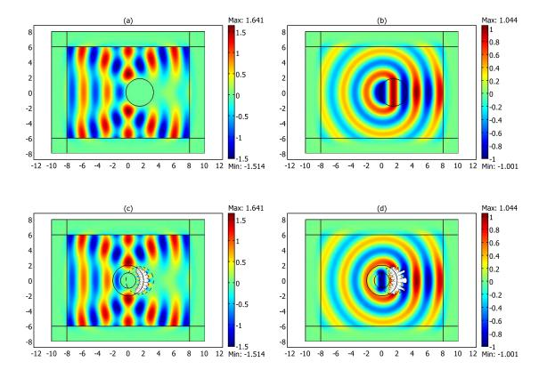
FIG. 2: (Color online) Snapshot of the total and scattering electric field. (a)-(b) The total and scattering electric field caused by a PEC cylinder with its outer boundary depicted by  $c = \rho_3(\theta)$ , respectively. (c)-(d) The total and scattering electric field induced by the designed PEC reshaper, respectively. The dashed lines in (c) and (d) outline the boundary of the effective PEC cylinder, which is the same to the outer boundary of the PEC cylinder in (a) and (b).
