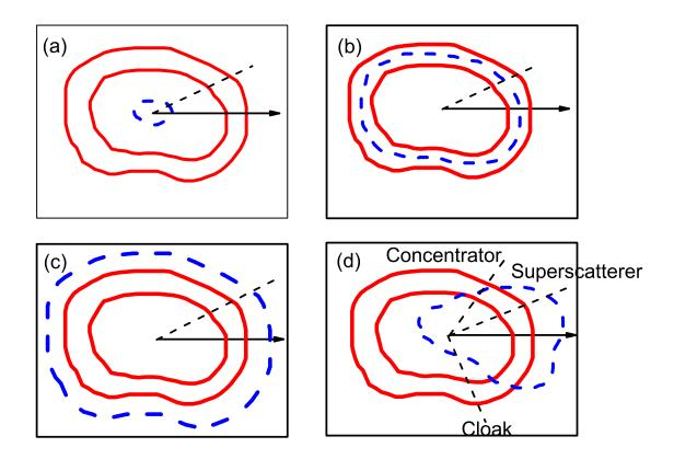
FIG. 1: (Color online) The schematic plot for the coordinate transformation of (a) an imperfect cylindrical cloak with arbitrary cross section, (b) a cylindrical concentrator with arbitrary cross section, (c) a cylindrical superscatterer with arbitrary cross section, and (d) a cylindrical PEC reshaper. The red solid lines denote the outer and inner boundaries of the above devices, while the blue dashed lines outline the effective PEC boundaries in the view of the outside world.
