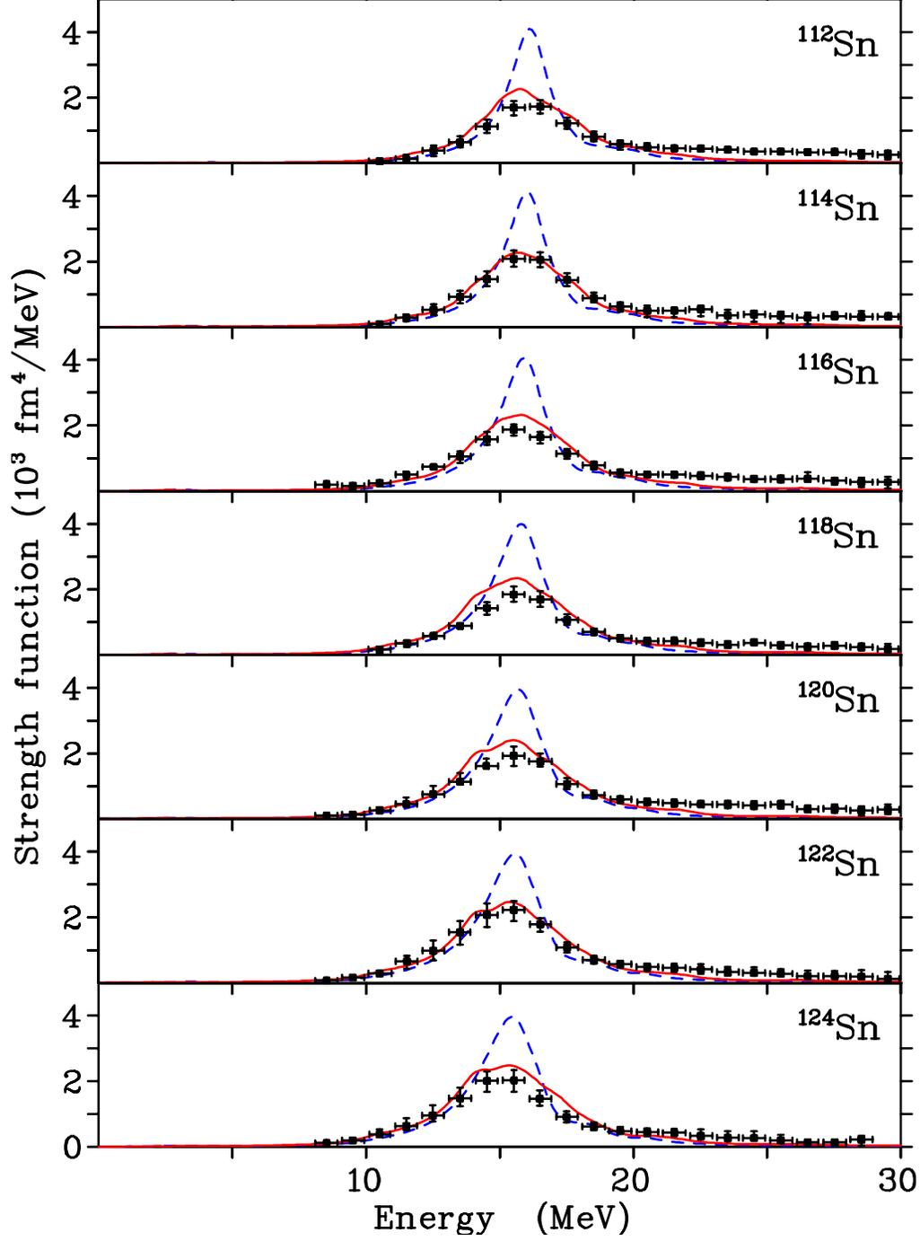
FIG. 1: Isoscalar giant monopole resonance in the even- $A$   $^{112-124}\text{Sn}$  isotopes calculated within QRPA (dashed line) and QTBA (solid line). The results are obtained within self-consistent HF+BCS approach based on the T5 Skyrme force. The smearing parameter  $\Delta$  is equal to 500 keV. Experimental data (solid squares) are taken from Ref. [18].
