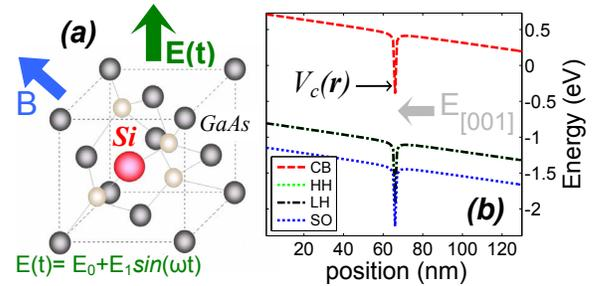
**FIG. 1** (a) Proposed geometry for  $g$ -tensor modulation. (b) The impurity potential is a Coulomb potential plus a central cell correction. The effect of applying an electric field on the zone center band energies is shown.
