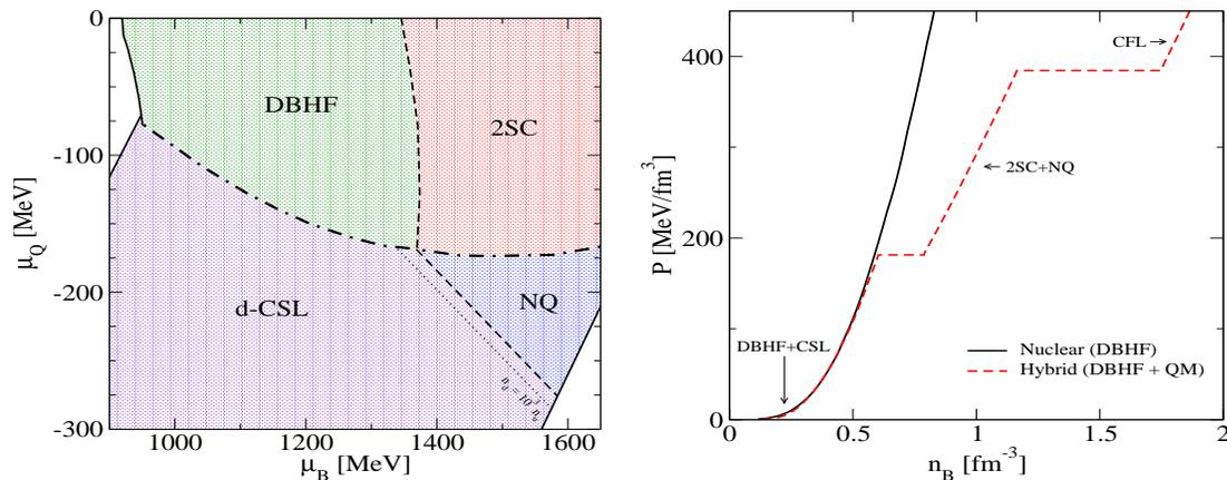
**Figure 1.** Left panel: Phase diagram in the plane of baryon and charge chemical potential. The dash-dotted line denote the border between oppositely charged phases. Right panel: Pressure of matter in  $\beta$ -equilibrium as a function of the density.
