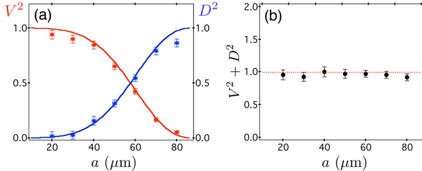
**Figure 5.** (a) Wave-like information  $V^2$  and particle-like information  $D^2$  as a function of the width  $a$  of the transmitting slits. The solid lines are the theoretical expectations given by equations (10) and (13) without any fitting parameter. (b)  $D^2 + V^2$  as a function of  $a$ .
