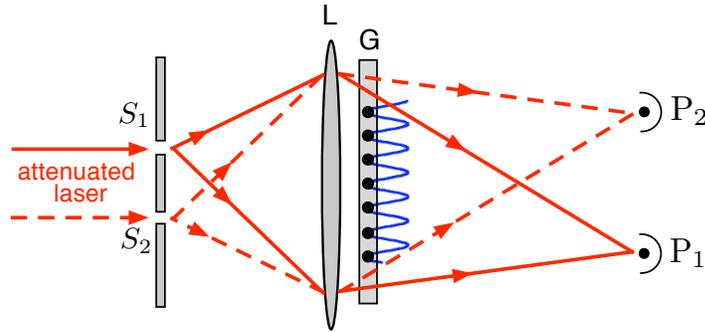
**Figure 1.** Simplified representation of Afshar’s experiment [28, 29]. An attenuated laser illuminates a Young’s double-pinhole interferometer. A lens (L) images each pinhole  $S_1$  and  $S_2$  on two detectors  $P_1$  and  $P_2$ . A grid of thin wires (G) with a period matching the interfringe is positioned after the lens so that the wires of the grid are exactly superimposed on the dark fringes of the interference pattern.
