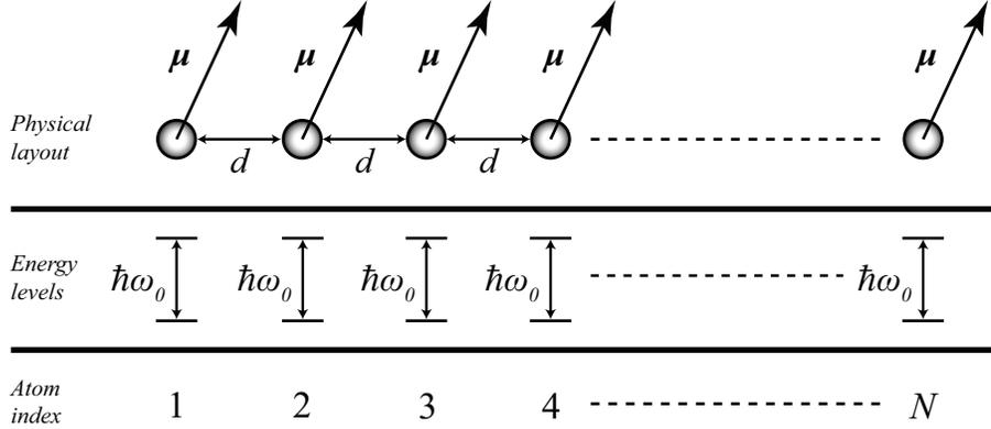
**Figure 1.** Physical layout of the linear chain. The atoms are equally separated from each other by a distance  $d$ , and are polarized in the same direction in their dipole moments  $\mu$  and their two-level energy structure (shown beneath each atom).
