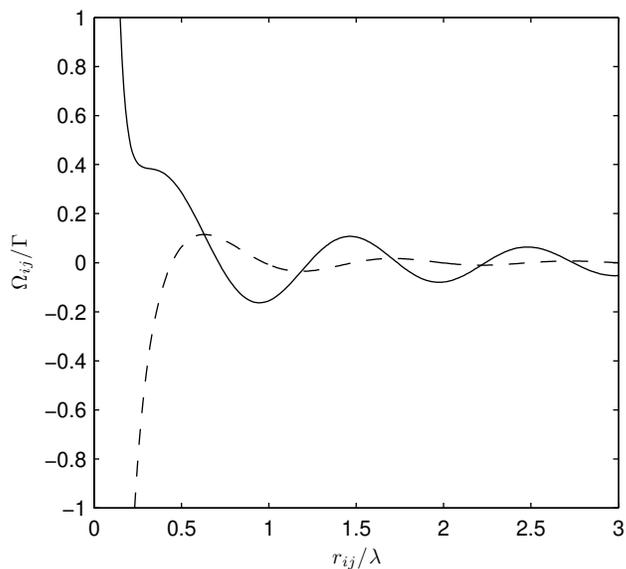
**Figure 2.** Dipole-dipole interaction strength as a function of  $r_{ij}/\lambda_0$  for two different orientations of the atomic dipole moments relative to the interatomic axis,  $\hat{\mu} \perp \hat{r}_{ij}$  (solid line) and  $\hat{\mu} \parallel \hat{r}_{ij}$  (dashed line).
