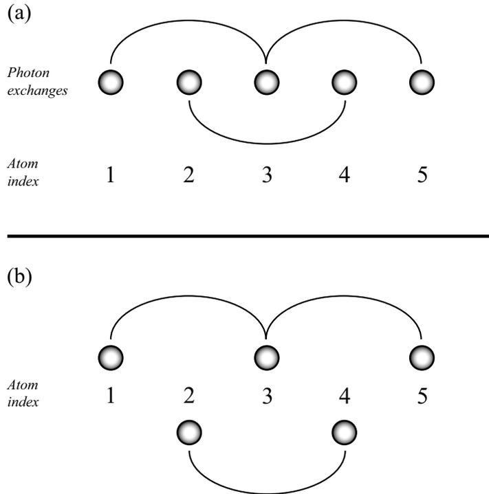
**Figure 4.** (a) Next-nearest-neighbour interactions in a five atom chain. (b) The chain is visually separated into its two subchains; the fact that no photon lines connect them means that they do not interact with one another.
