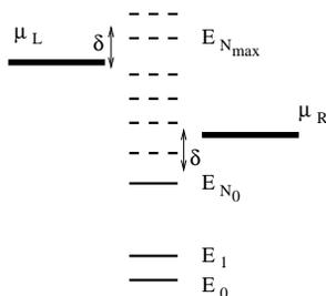
**Figure 2.** The initial configuration in the many-level quantum dot for a given pair of chemical potentials on the leads  $\mu_L, \mu_R$  and a 'gap'  $\delta$ . The occupied levels are marked by thick lines.
