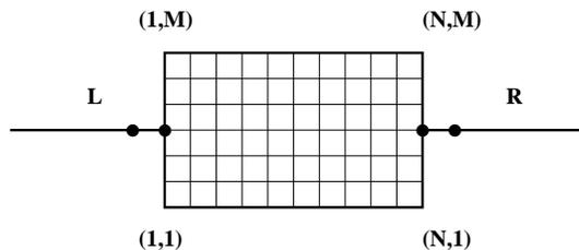
**Figure 1.** A schematic picture of the system we have studied. Two (semi-infinite) one-dimensional leads are attached to a two-dimensional sample described by a  $N \times M$  sites. The solid dots indicate the contact sites; each site  $i$  of the sample is characterized by two indices  $(x_i, y_i)$  where  $x_i = 1, \dots, N$  and  $y_i = 1, \dots, M$ .
