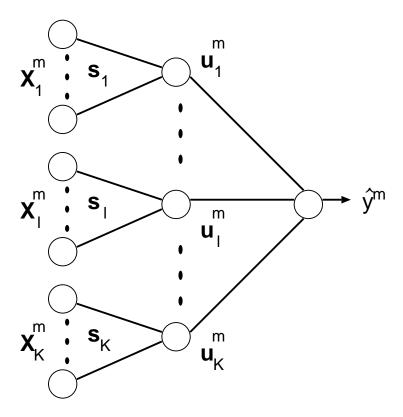
FIG. 2: General architecture of the treelike multilayer perceptron with N input units and K hidden units.
