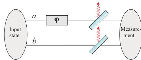
FIG. 1: General optical interferometric setup with two arms. Channel  $a$  acquires a phase  $\varphi$  relative to channel  $b$ . The two beam splitters in channel  $a$  and  $b$  symbolize photon losses.
