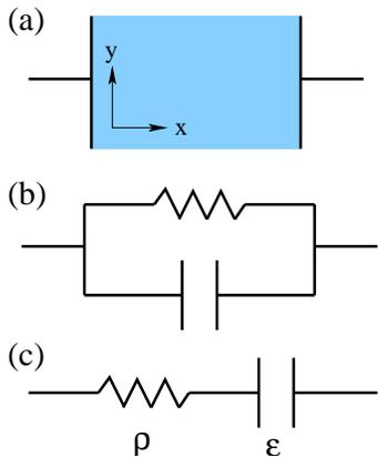
FIG. 1: Simple circuits of resistors  $\hat{\rho} \equiv \hat{\sigma}^{-1}$  and capacitors  $\varepsilon$  that illustrate the basics of dielectric response. Diagram (a) depicts the measuring set-up, where a rectangular sample is confined between metallic plates and subjected to an applied electric field  $E_x \hat{x}$ , (b) represents a simple homogeneous medium, and (c) represents the simplest metal-insulator composite that exhibits the Maxwell-Wagner effect.
