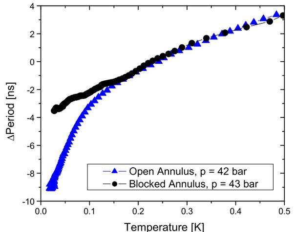
FIG. 3: Resonance period as a function of temperature in an open (solid triangles) and blocked (solid circles) annulus with a width of  $73.4 \mu\text{m}$ . Both open and blocked annulus data are taken in the same cell which could be reversibly blocked (see Fig. 1). The nonclassical rotational inertia decoupling is 17.1% of the solid inertia in the open annulus. For the blocked annulus, the upper limit to the NCRI is 0.8% corresponding to a more than twentyfold reduction upon blocking.
