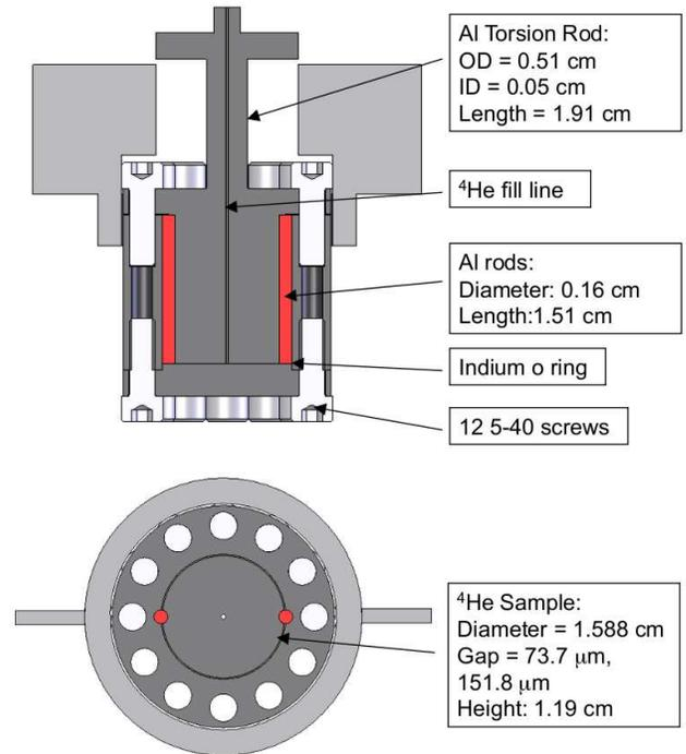
FIG. 1: Aluminum torsional oscillator with removable blocks (in red). The thin annular gap widths of  $73.4 \mu\text{m}$  and  $148.3 \mu\text{m}$  resulted in mass loading of 45.5 ns and 91.9 ns respectively. At 20 mK, the resonance frequency is 484.1 Hz and the quality factor of the oscillation is  $Q \sim 5.3 \times 10^5$ .
