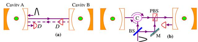
FIG. 6: (Color online) (a) Quantum state transfer from cavity A to cavity B. (b) Creation of entanglement between two atomic memories. Where D, PBS, C, BS, and M denote single photon detector, polarizing beam splitter, circulator, 50/50 beam splitter, and mirror, respectively.
