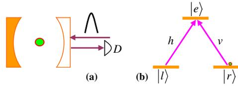
FIG. 1: (Color online) (a) Schematic setup to reflect a single photon pulse from one-sided cavity. (b) The relevant atomic level structure and transitions.
