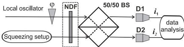
FIG. 1: The scheme of the HD setup. The beam from the squeezing setup is interfering with the LO on a 50/50 beam-splitter **BS**,  $\phi$  is the phase of the LO, **D1** and **D2** are analogue photodetectors. Linear attenuation is introduced in both beams by the neutral density filter **NDF**. The produced photocurrents  $i_1$  and  $i_2$  are further analyzed by the computer.
