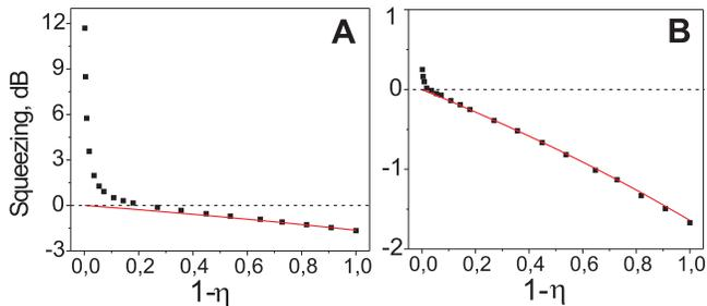
FIG. 3: Experimental dependence of the squeezing on the transmission  $1 - \eta$ : (A) for the subtraction method and (B) for the covariance method. Red solid line represents the theoretical dependence without accounting for the EN. Horizontal dashed line at zero defines a border between the squeezing and the classical access noise.
