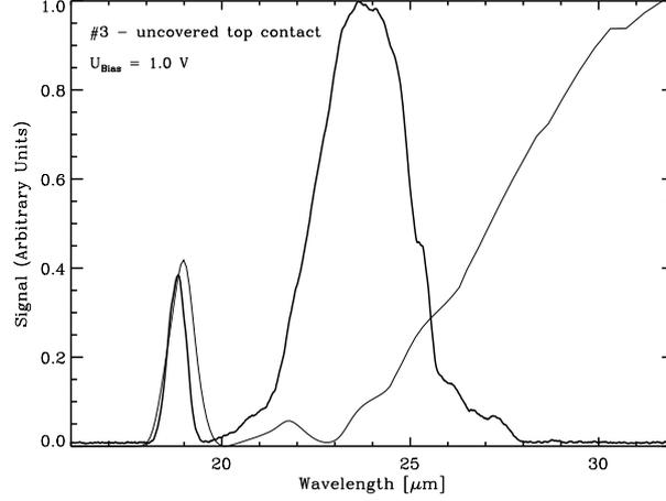
Figure 6. The normalized detector signal (thick line) for the wavelength range  $16\mu\text{m} \leq \lambda \leq 32\mu\text{m}$  when illuminated through a cut-on filter. The transmission of the filter is denoted by the thin line. Because there was no reference detector (bolometer) for this measurement, the BIB detector signal was not corrected neither for the grating efficiency, atmospheric transmission, nor the black body spectrum.
