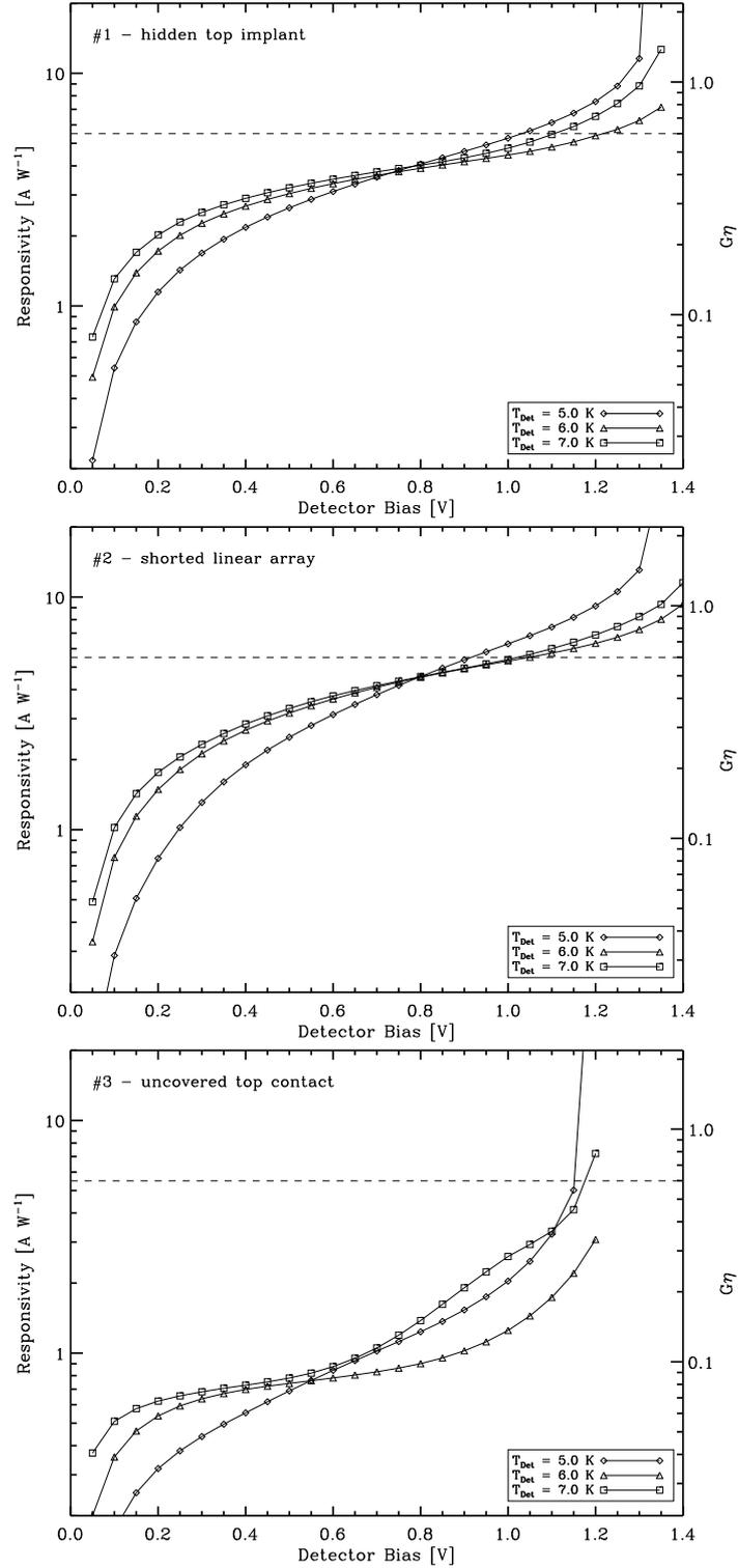
Figure 7. Responsivity (left scale) and the quantum efficiency photoconductive gain product  $G\eta$  (right scale) of the three tested detectors for three temperatures and in dependence of the bias voltage, measured at a wavelength of  $\lambda = 11.3 \mu\text{m}$ .
