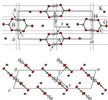
**Figure 1.** Schematic view of the crystalline structure of  $\text{KHCO}_3$  at 300 K. The arrows point to the sites occupied at low temperature (the  $L$  configuration, see text). Dashed lines through protons are guides for the eyes. The ellipsoids represent 50% of the probability density for nuclei.
