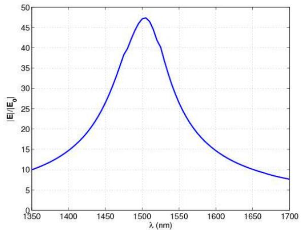
FIG. 5: Maximum field enhancement,  $|E|/|E_0|$ , in the PIMNIM vs. wavelength. It is noted that the enhancement is maximized at the absorption peak, and has no structure corresponding to the electric resonance at  $\lambda = 1380$  nm.
