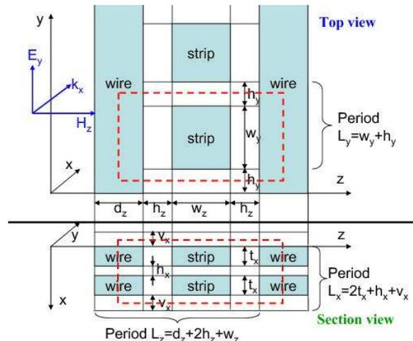
FIG. 2: (Color online) Schematic of the PIMNIM structure. Unit cell for electromagnetic and electrostatic simulations is inside the dashed rectangles.
