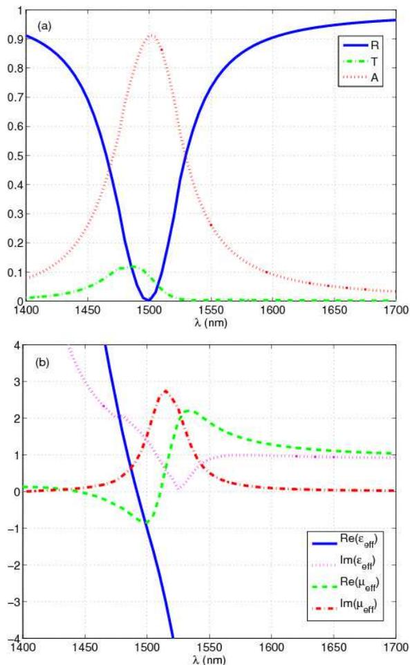
FIG. 4: (Color online) (a) Reflectance, transmittance and absorbance at normal incidence of a single PIMNIM layer. (b) Extracted effective dielectric permittivity  $\epsilon_{\text{eff}}$  and magnetic permeability  $\mu_{\text{eff}}$  of the PIMNIM structure. Reflectance vanishes at  $\lambda = 1.5 \mu\text{m}$  because  $\epsilon_{\text{eff}} = \mu_{\text{eff}}$ . Parameters (in nm):  $L_y = 326$ ,  $w_y = 208$ ,  $t_x = 80$ ,  $w_z = 46$ ,  $d_z = 78$ ,  $h_x = 21$ ,  $h_z = 20$ .
