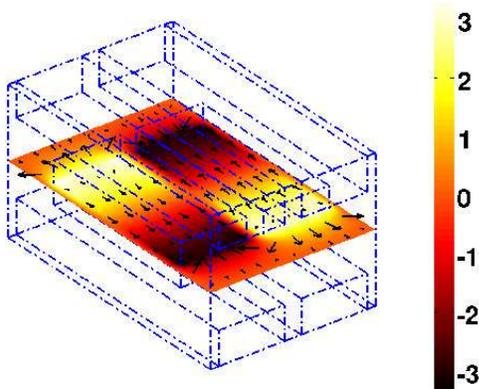
FIG. 3: (Color online) Electrostatic magnetically-active plasmon resonance of the PIMNIM structure shown in Fig. 2 with the scalable geometric proportions corresponding to (in nm):  $L_y = 320$ ,  $w_y = 200$ ,  $t_x = 80$ ,  $w_z = 50$ ,  $d_z = 80$ ,  $h_x = 20$ ,  $v_x = 10$ ,  $h_z = 20$ . The resonance occurs at  $\epsilon_m/\epsilon_d = -26.8$ . Arrows: electric field; color: electrostatic potential.
