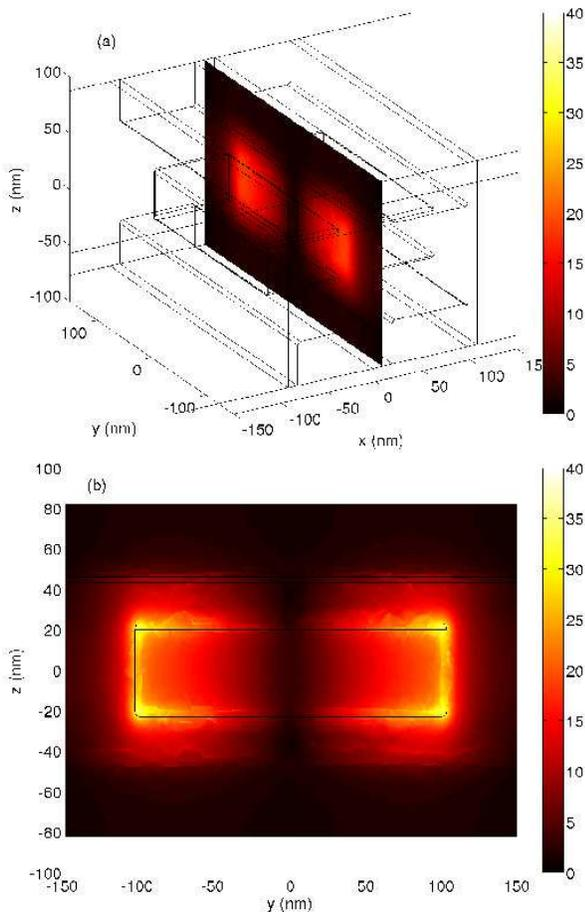
FIG. 6: (Color online) Field enhancement,  $|\mathbf{E}|/|E_0|$  in the PIMNIM. Field is plotted on  $y-z$  slices at (a)  $x = 0$  and (b)  $x = -8$  nm. Although the largest enhancement is near the edges and corners, a relatively large area experiences significant enhancement.
