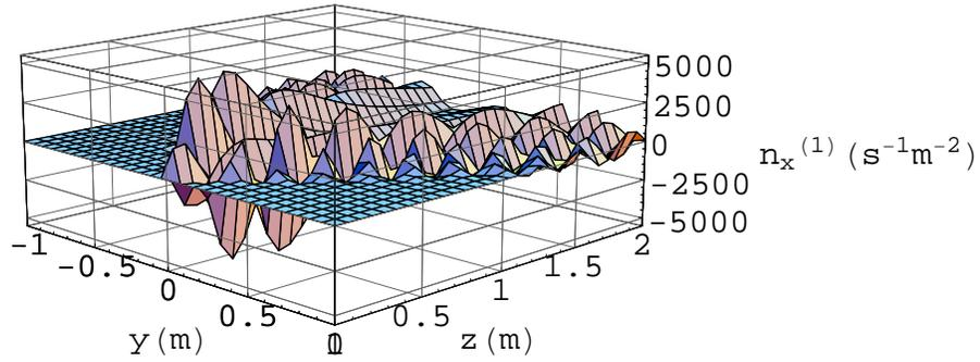
Figure 3:  $n_x^{(1)}$  as a function of  $(y, z)$  on the plane  $x = 0.05$  m. The parameters are taken as  $A_{\otimes} \sim 10^{-30}$ ,  $\psi_0 = 1.8 \times 10^4$  V m $^{-1}$ ,  $W_0 = 0.05$  m,  $\hat{B}_y^{(0)} = 3$  T, and  $l = 0.4$  m for demonstration.
