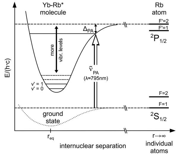
FIG. 1: Relevant level structure (not to scale) in the Rb atom and the YbRb\* molecule close to the D1-line of Rb at 795 nm. The detuning from resonance in wavenumbers is defined as  $\Delta_{\text{PA}} = \tilde{\nu}_{\text{PA}} - 12578.862 \text{ cm}^{-1}$ .
