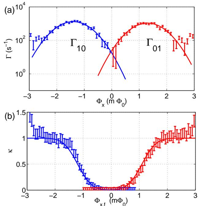
FIG. 3: (a) First MRT peaks in  $\Gamma_{01}$  and  $\Gamma_{10}$  and their best fit with Eq. (4). (b) The experimental value of  $\kappa$  as defined in (8) as a function of the final bias  $\epsilon_f$ . The solid line shows the theoretical curve (10) using the parameters obtained from the best fit in (a).
