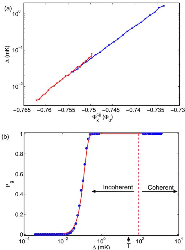
FIG. 4: (a) Plot of  $\Delta$  vs. flux bias  $\Phi_x^{cjj}$  applied to the compound junction. The lower curve is  $\Delta$  measured with MRT and the upper curve is  $\Delta$  measured with LZ. (b) Experimental (dots) and theoretical (line) ground state probability  $P_g = 1 - P_{LZ}$ , for fixed  $\nu = 0.05\Phi_0/\mu s$  as a function of  $\Delta$ . The dashed line indicates the crossover between the incoherent and coherent regime, defined by  $W \approx \Delta$ .
