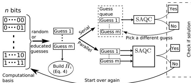
FIG. 5: (Color online) Implementation of an SAQC algorithm either in parallel or in serial.
