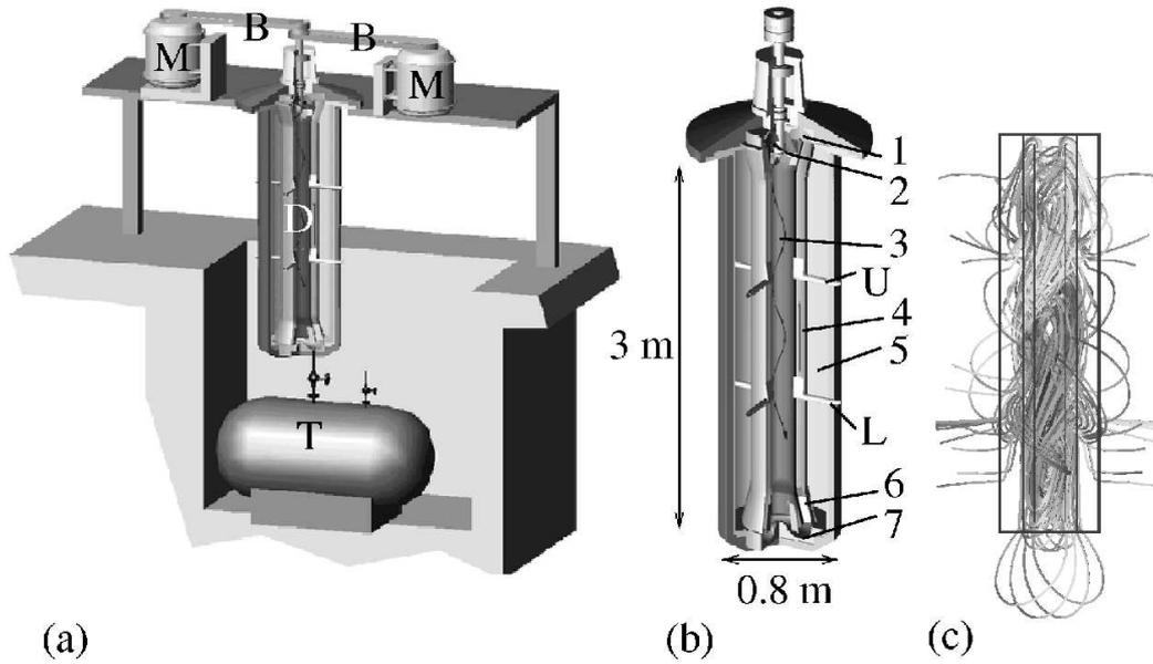
**Fig. 5** The Riga dynamo experiment and its eigenfield. (a) Sketch of the facility. M - Motors. B - Belts. D - Central dynamo module. T - Sodium tank. (b) Sketch of the central module. 1 - Guiding blades. 2 - Propeller. 3 - Helical flow region without any flow-guides, flow rotation is maintained by inertia only. 4 - Back-flow region. 5 - Sodium at rest. 6 - Guiding blades. 7 - Flow bending region. (c) Simulated magnetic eigenfield. The gray scale indicates the vertical component of the field.
