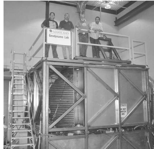
**Fig. 20** The rotating 3m sphere in Maryland. An impressive video is available under [www.youtube.com](http://www.youtube.com). Figure courtesy of D. Lathrop.
