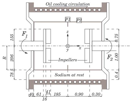
**Fig. 12** Design of the VKS experiment with two disks counter-rotating in the cylinder driving two poloidal and two toroidal eddies ( $s2^+t2$ ). The numbers on the l.h.s are the dimension in mm, the numbers on the r.h.s are the dimensions normalized by the radius. Figure courtesy of the VKS team.
