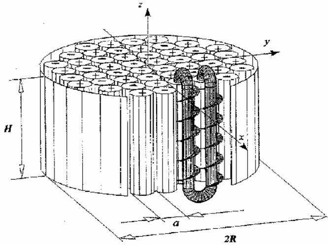
**Fig. 8** Central part of the Karlsruhe dynamo facility. The module consists of 52 spin-generators, each containing a central tube with non-rotating flow and an outer tube where the flow is forced on a helical path. Figure courtesy of R. Stieglitz.
