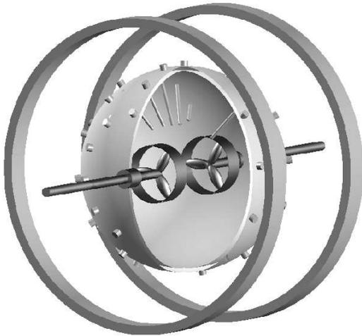
**Fig. 14** Schematic plot of the Madison Dynamo experiment (MDX). The flow topology is of the same  $s_2+t_2$  type as in the VKS experiment. The two rings symbolize the Helmholtz coil for producing an axial magnetic field. The lances for internal magnetic field sensors are also shown. Figure courtesy of E. Spence.
