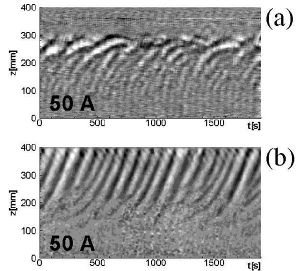
**Fig. 26** The measured axial velocity perturbation for  $Re = 2975$  and  $I_{coil} = 50$  A, showing the appearance of MRI as a travelling wave. (a) PROMISE 1 experiment with  $I_{rod} = 6000$  A. (b) PROMISE 2 experiment with  $I_{rod} = 7000$  A.
