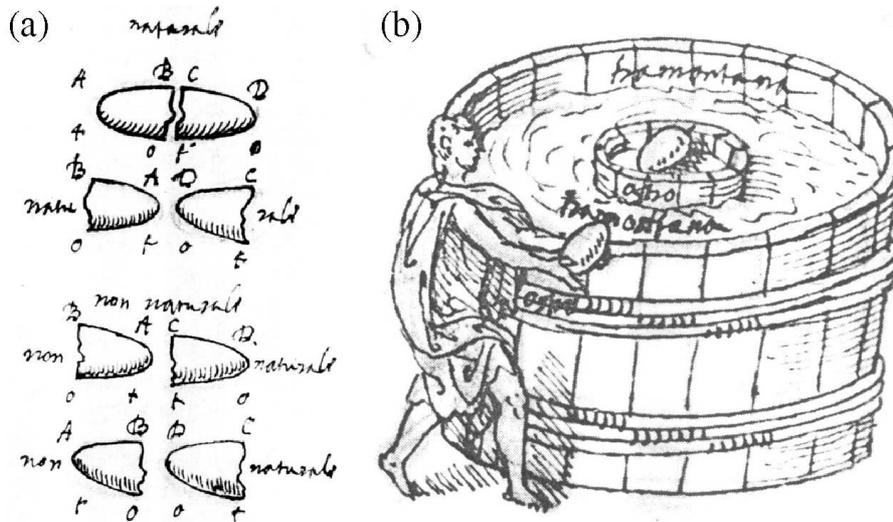
**Fig. 1** Lodestone experiments of Petrus Peregrinus. (a) Experiments showing the attracting and repelling forces of a broken piece of lodestone. Upper configuration: "naturale", lower configuration: "non naturale". (b) A simple compass. Figures from [169].
