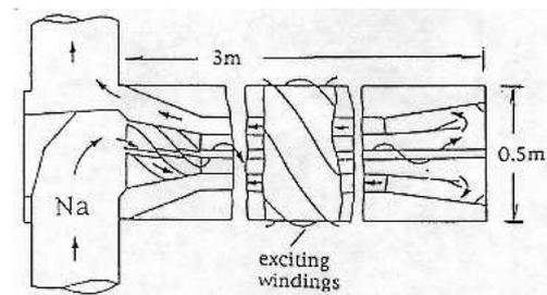
**Fig. 4** The dynamo module of the 1987 experiment. Significant amplifications of externally applied magnetic fields were measured, before the experiment had to be stopped due to mechanical vibrations.
