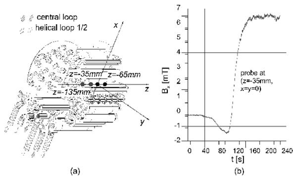
**Fig. 10** Self-excitation and saturation in the Karlsruhe dynamo experiment. (a) The dynamo module with the connections between the spin-generators and the supply pipes. (b) Hall sensor signals of  $B_x$  in the inner bore of the module. Figure courtesy of R. Stieglitz.
