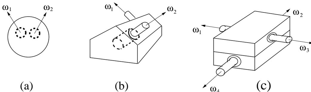
**Fig. 2** (a) The Herzenberg dynamo. Two spheres rotate around non-parallel axes. (b) The first dynamo of Lowes and Wilkinson. Two cylinders rotate in a “house-shaped” block. (c) The fifth dynamo with four independent rotors.
