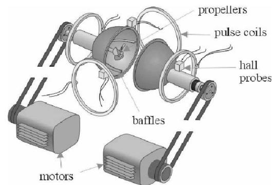
**Fig. 18** The second dynamo experiment in Maryland. In a 0.3 m diameter sphere different flows have been produced by propellers. This configuration, but with the propellers replaced by an inner sphere, was used for the MRI experiment. Figure courtesy of D. Lathrop.
