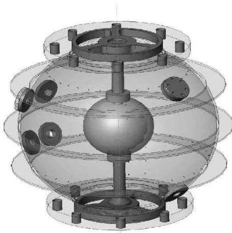
**Fig. 21** The DTS experiment in Grenoble. Forty liters of liquid sodium are contained between a 7.4 cm inner sphere and a 21 cm radius outer sphere. The copper inner sphere contains a magnet which produces a nearly dipolar field with a maximum of 0.345 T in fluid close to the poles. Figure courtesy of D. Schmitt and the DTS team.
