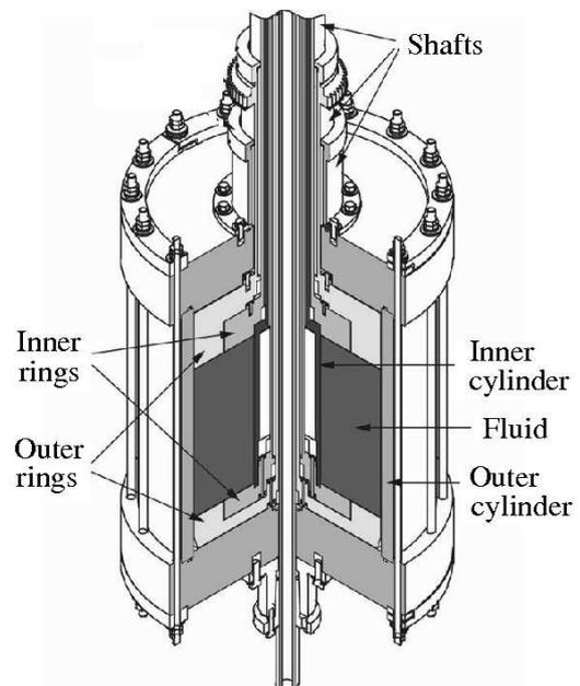
**Fig. 22** The Princeton MRI experiment. The rotating gallium of height 27.86 cm is contained between two differentially rotating concentric cylinders of radii 7.06 cm and 20.30 cm. Figure courtesy of H. Ji.
