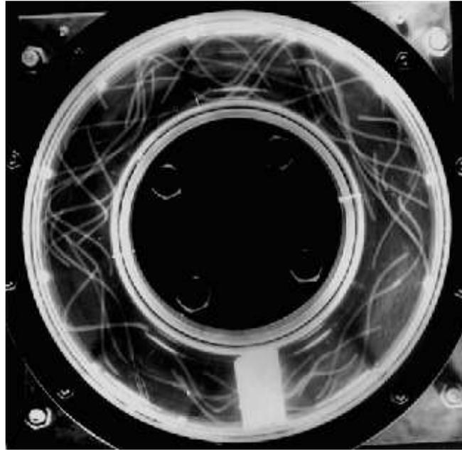
**Fig. 16** Helical flow that develops after the abrupt brake of the torus in the Perm water test experiment, visualized by polystyrene particles. The white bar at the bottom of the picture represents the diverter. Figure courtesy of P. Frick.
