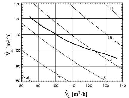
**Fig. 11** Isolines of the dimensionless number  $C = \mu_0 \sigma \alpha_{\perp} R$  in the  $\dot{V}_C - \dot{V}_H$ -plane. In a certain approximation, dynamo action should occur beyond the isoline with  $C_{crit} = 8.12$  [176]. The experimentally determined neutral line (bold), separating regions with and without dynamo action, slightly deviates from the theoretical line. Figure courtesy of K.-H. Rädler.
