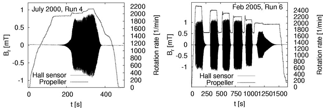
**Fig. 6** Two experimental runs carried out in July 2000 and in February 2005. Rotation rate of the motors, and magnetic field measured at one Hall external sensor plotted vs. time. After the exponential increase of the magnetic field in the kinematic dynamo regime, the dependence of the field level on the rotation rate has been studied in the saturation regime.
