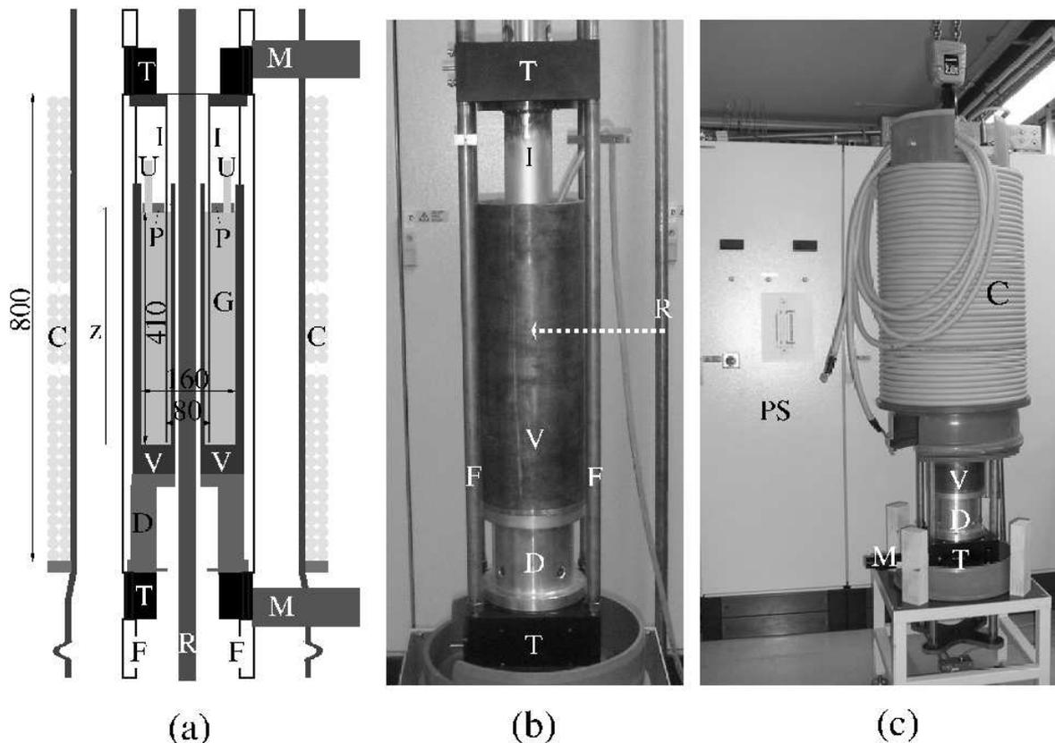
**Fig. 24** The PROMISE experiment. (a) Sketch. (b) - Photograph of the central part. (c) - Total view with the coil being installed. V - Copper vessel, I - Inner cylinder, G - GaInSn, U - Two ultrasonic transducers, P - Plexiglas lid, T - High precision turntables, M - Motors, F - Frame, C - Coil, R - Copper rod, PS - Power supply for currents up to 8000 A. The indicated dimensions are in mm.
