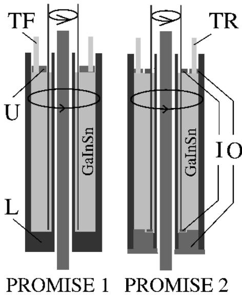
**Fig. 25** The asymmetric end cap configuration in PROMISE 1 is replaced by a symmetric one in PROMISE 2. U - Upper end cap fixed in the laboratory frame, L - Lower end cap, made of copper, rotating with the outer cylinder, I - Inner plastic rings, O - Outer plastic rings, TF - Fixed ultrasonic transducer, TR - Rotating ultrasonic transducer.
