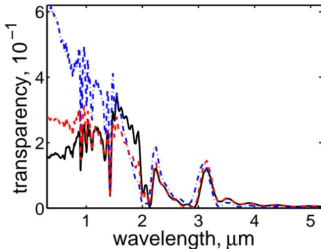
FIG. 6: (Colour online) Transmission through a 800 nm hole-size lattice when the film is illuminated by a plane wave (solid line), Gaussian beam waist size 1  $\mu\text{m}$  (dashed dotted line) and 2  $\mu\text{m}$  (dashed line). Source focal planes are located at 1.4  $\mu\text{m}$  from the gold surface.
