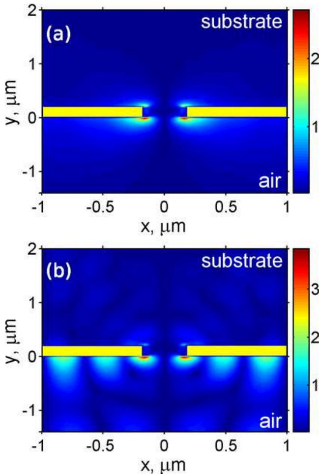
FIG. 4: (Colour online) Calculated amplitude distribution of  $Z$  component of electrical field in simulation for a single hole (a) and periodical lattice of holes (b). The cross section is made at the center of hole. Light source is polarized along  $X$ ,  $\lambda = 0.7 \mu\text{m}$ .
