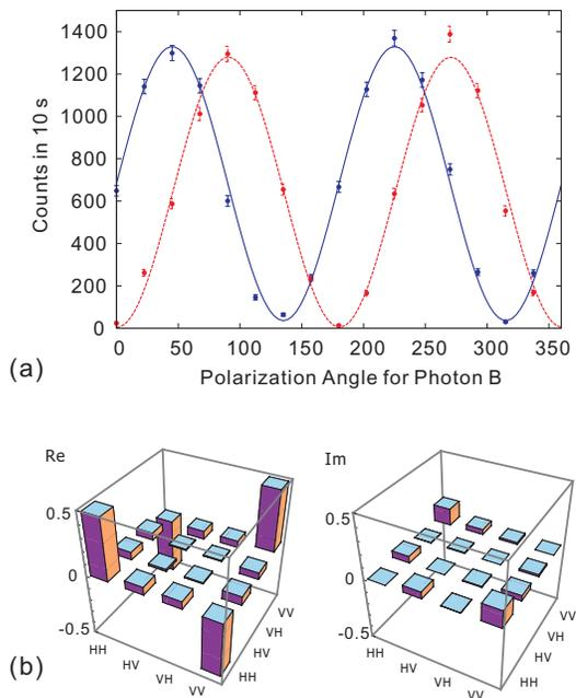
FIG. 2: (color online). (a) Polarization correlations for the entangled photon pair. Polarization angle for photon A is fixed to  $90^\circ$  for the red, and  $-45^\circ$  for the blue. Error bars represent statistical errors. (b) Tomography measurement result, with the left for the real part, the right for the imaginary part.
