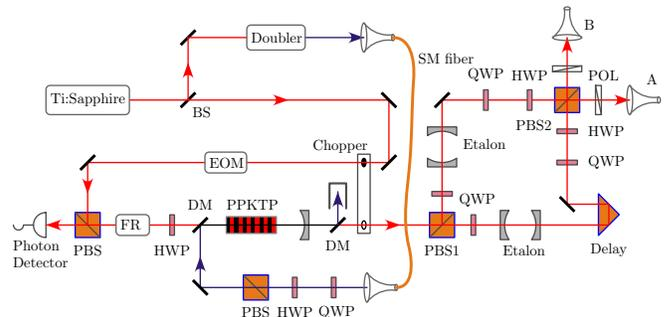
FIG. 1: (color online). Layout of the experiment. The generation of polarization entanglement is realized by interfering the two down-converted photons on PBS2. An electro-optic modulator (EOM) phase modulated at 70 MHz is utilized to generate sidebands for the locking beam. A PBS, a Faraday rotator (FR) and a half-wave plate (HWP) is utilized to extract the reflection beam and to generate the error signal for the locking system.
