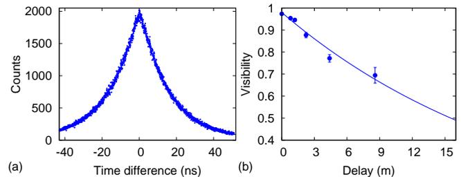
FIG. 3: (color online). (a) Time correlation measurement. The data is fitted with a function of  $c_0 e^{-2\pi\Delta\nu|t|}$ . The FWHM correlation time is 23.0 ns. (b) Visibility in  $|+\rangle/|-\rangle$  basis as a function of the relative delay. The data is fitted with a function of  $v_0 e^{-x/x_0}$ . Error bars represent statistical errors.
