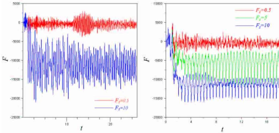
**Figure 8.** Time dependencies of the friction force for films with thickness of one (left) and two (right) molecular diameters and different driving forces. The value of load is 50. Negative trend is the consequence of the fact that friction force acts in the direction reverse to sliding.
