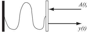
Figure 3: A Fabry-Perot optical cavity. The black rectangle denotes a mirror fully reflecting at the cavity resonance frequency while the white rectangle denotes a mirror partially transmitting at that frequency.
