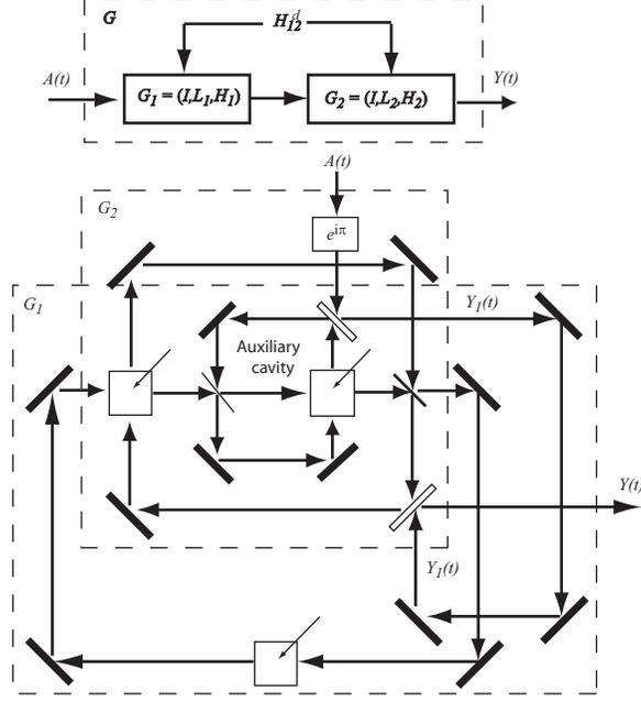
Figure 20: Realization of  $G$ . The block diagram at the top shows how  $G$  is realized by a series connection of  $G_1$  into  $G_2$  and a bilinear direct interaction  $H_{12}^d$  between the canonical operators of  $G_1$  and  $G_2$ . The bottom figure shows the physical implementation of  $G$  based on the block diagram
