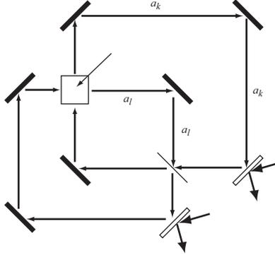
Figure 17: Example implementation of the total direct interaction  $H_{kl} = H_{kl}^1 + H_{kl}^2$  between the modes  $a_k$  and  $a_l$  of two ring cavities
