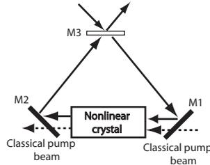
Figure 7: A degenerate parametric amplifier consisting of a classically pumped nonlinear crystal in a three mirror ring cavity
