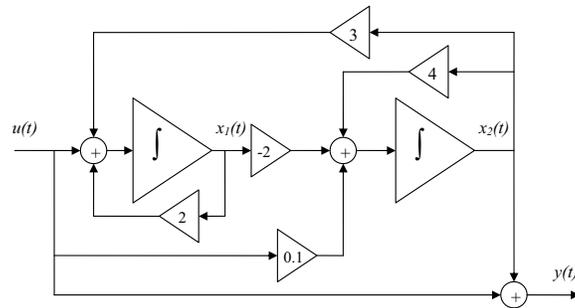
Figure 1: Schematic for the implementation of the classical system (1.1).
