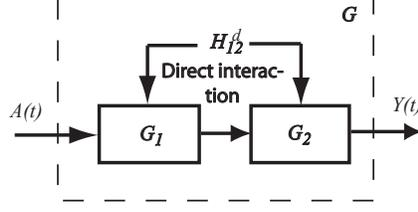
Figure 5: Cascade connection of  $G_1$  and  $G_2$  with indirect interaction  $H_{12}^d$
