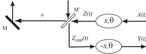
Figure 16: Scheme for implementation of a coupling  $L = \tilde{\alpha}a + \tilde{\beta}a^*$  with  $\tilde{\alpha} > 0$  and  $\tilde{\alpha} > |\tilde{\beta}|$ . Here  $s = -\text{arccosh}(\tilde{\alpha}/\sqrt{\gamma})$ ,  $\theta = \arg(\tilde{\beta})$  and the mirror  $M'$  has coupling coefficient  $\gamma = \sqrt{\tilde{\alpha}^2 - |\tilde{\beta}|^2}$
