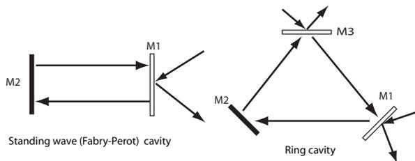
Figure 6: Two types of optical cavities: a standing wave or Fabry-Perot cavity (left) and a (three mirror) ring cavity (right). Arrows indicate the direction of propagation of light in the cavity. Black rectangles denote fully reflecting mirrors while white rectangles denote partially transmitting mirrors.
